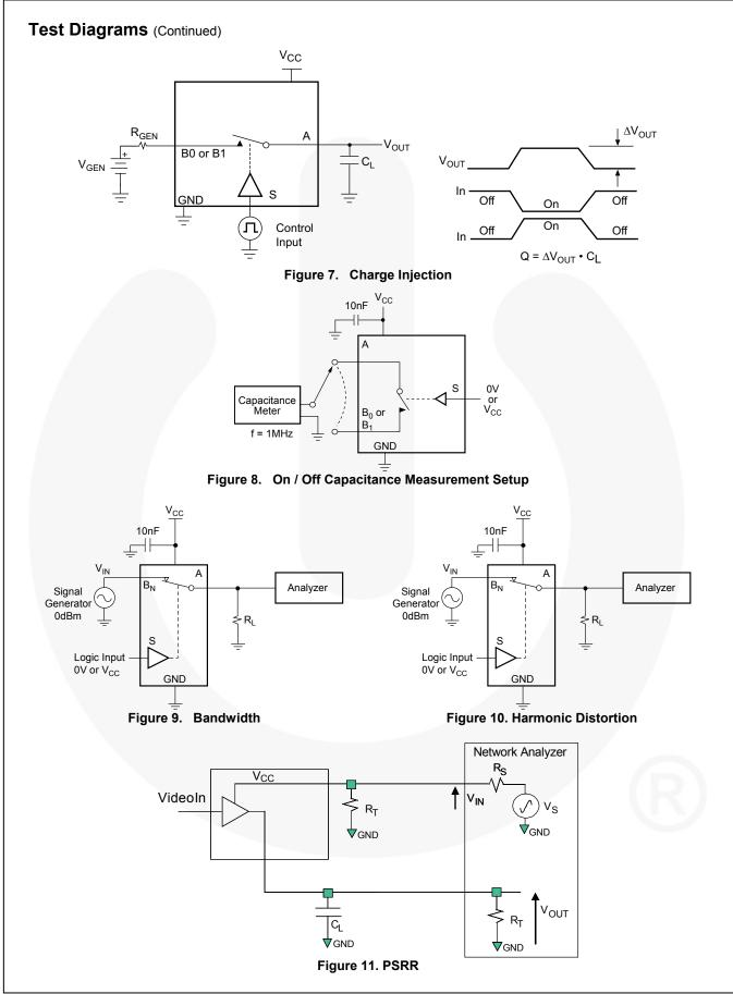
FSA839 — Low-Voltage, 0.8Ω SPDT Analog Switch with Power-Off Isolation
