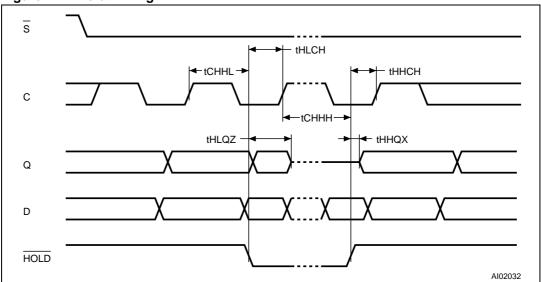
Figure 25. Output Timing
