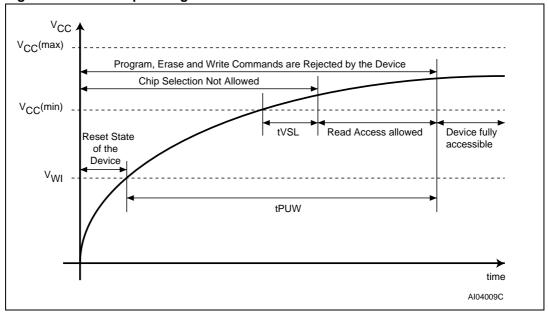
Table 8. Power-Up Timing and VWI Threshold
