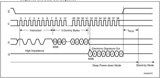
1. The value of the 8-bit Electronic Signature, for the M25P40, is 12h.
