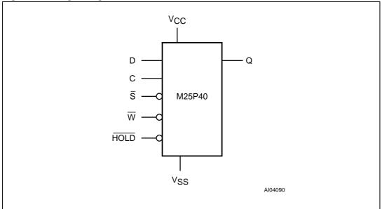
Figure 2. SO and VFQFPN Connections
