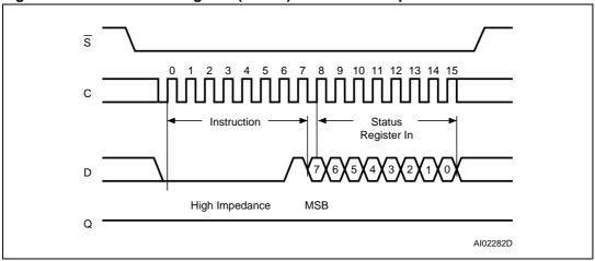
Figure 11. Write Status Register (WRSR) Instruction Sequence
